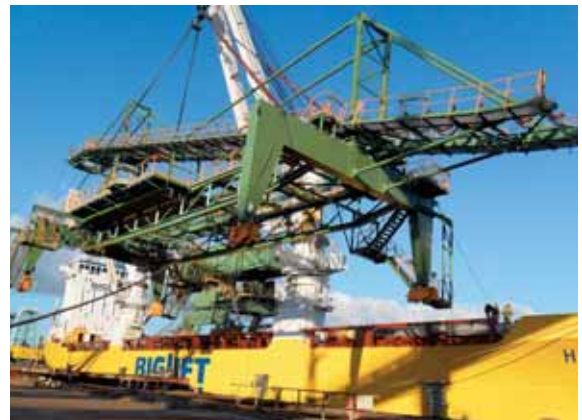
Conveyor element loaded on a "heavy lift" ship by an expedition heading towards Antipodes
