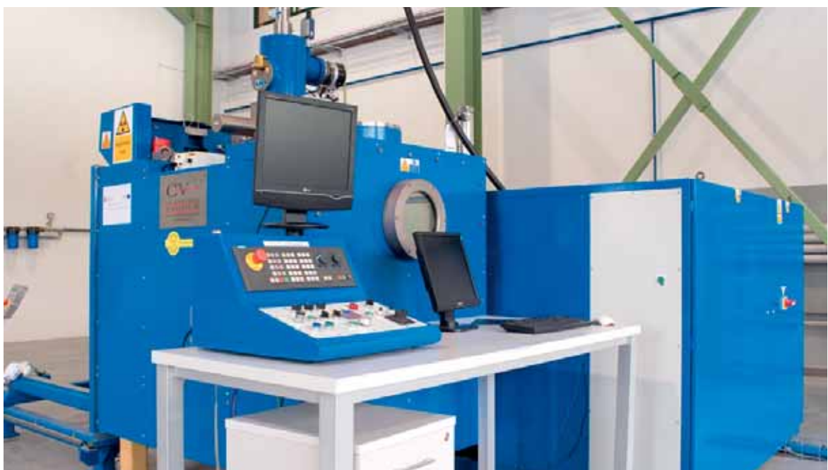
CVE SC8-5209 electron beam welding device (Vertical Machining Center MAZAK VTC 800/30 SR)
