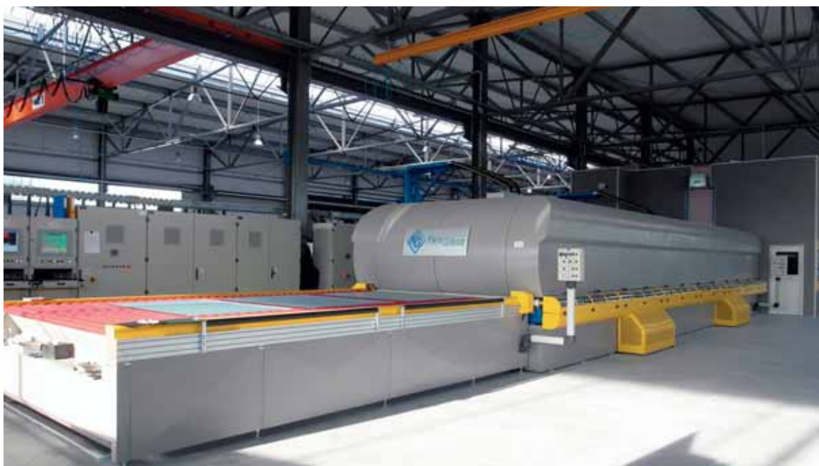
Line used to pre-stressing of construction glass
