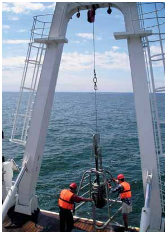
The collection of surface sediments with the use of Box Cover device to geological research of Southern Baltic Sea
