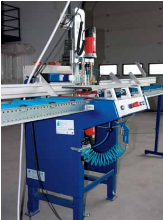
Vertical drill to simultaneous, co-axial performance of holes in guides
