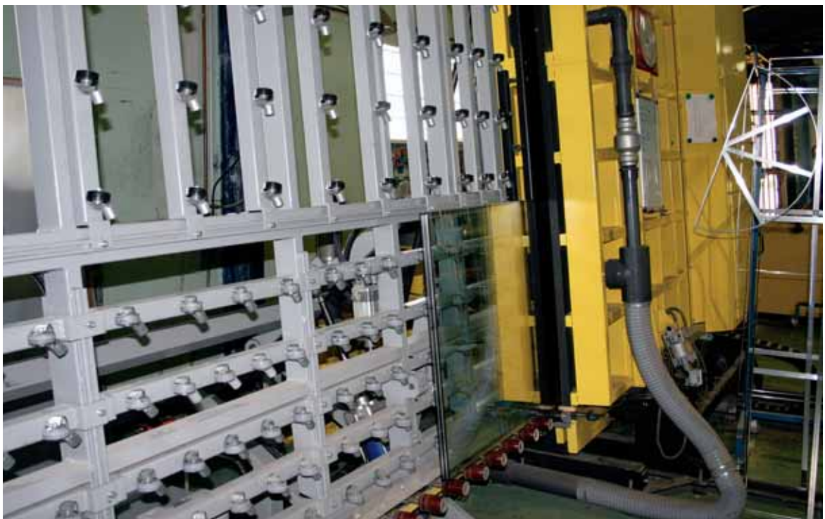
Production of insulated glass
